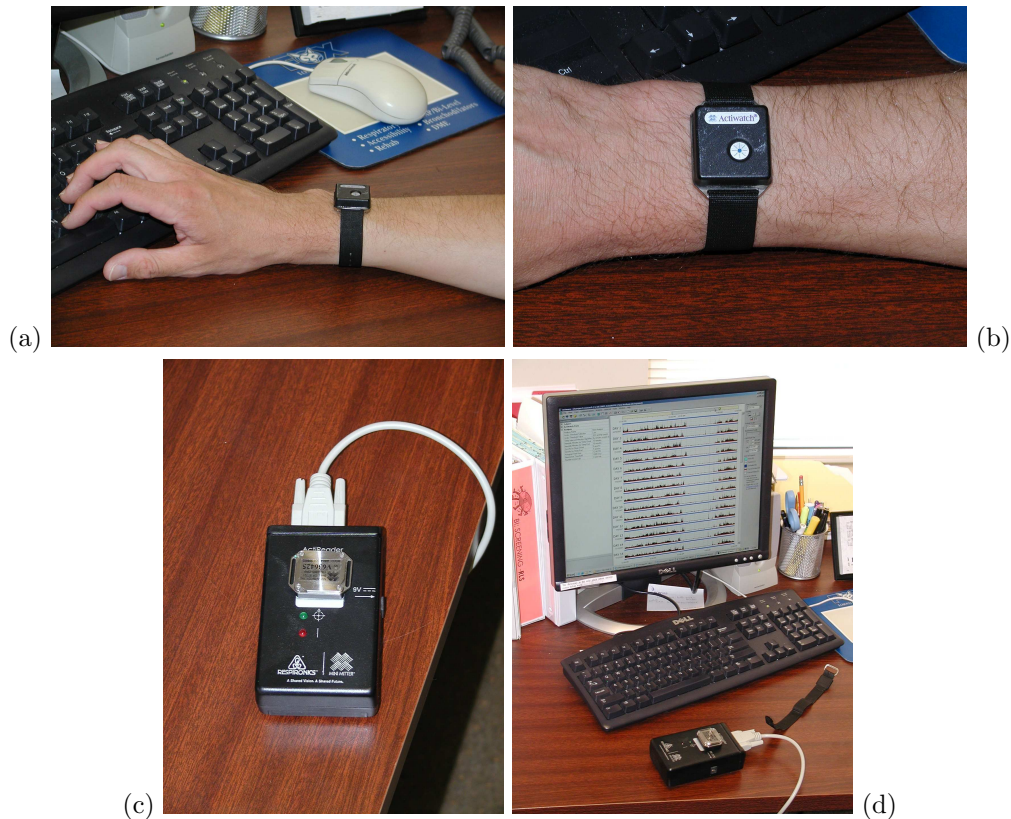
Figure 1: (a) What looks like a regular watch from the distance turns out to be an actigraph (b), here an Actiwatch from Respironics, Inc. (c) Via an ActiReader device from Respironics, Inc., data is transferred every few weeks from the Actiwatch to a computer where it is stored and (d) displayed on the computer screen.
